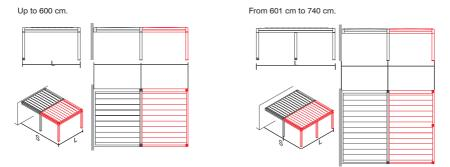
The extension of the TYPE 1 coupled module is considered from the leg axis of the base module to the outer leg of the coupled module.
