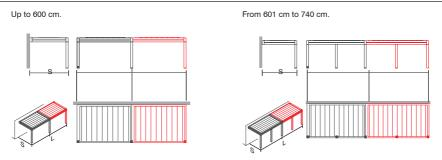
The width of the TYPE 2 coupled module is different than the extension of the base module because the coupled module does not consider the overall 17 cm dimensions of the coupling leg. The width of the TYPE 2 coupled module is considered from the leg axis of the base module to the outer leg of the coupled module.
