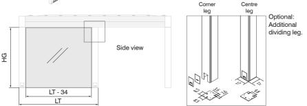
Side drop awnings can be assembled on a AZIMUT structure already installed.
