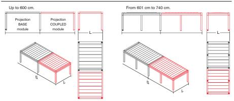
The extension of the TYPE 2 coupled module is different than the extension of the base module because the coupled module does not consider the overall 17 cm dimensions of the coupling leg. The extension of the TYPE 2 coupled module is considered from the leg axis of the base module to the outer leg of the coupled module.
