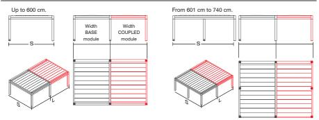
The width of the TYPE 1 coupled module is considered from the leg axis of the base module to the outer leg of the coupled module.
