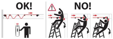
The opening and closing of the motorized awning can be performed thanks to a switch, installed in the vicinity of the awning and in a position such as to allow the user the total visibility of its movements (if placed outdoor, the switch must be suitably protected) or, in the case of radio engines, using a portable or wall mounted radio control (see sec. 6.3) or wall (the awning must be operated from a site able to guarantee a good visibility of the excursion of the fabric cover).
