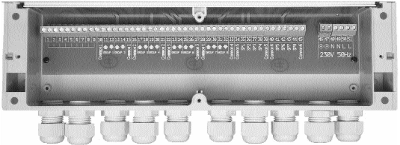
The mains power supply (230 V~, 50 Hz) for the device must be made on the connections 46 to 51. The connections 1 to 9 are internally connected and can be used for example to connect the minus of the 24 Volt.
