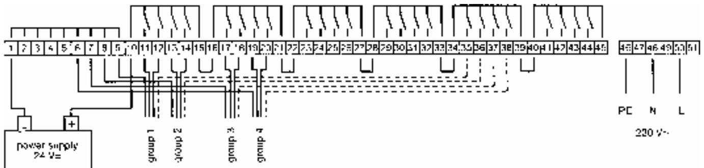
**Note:** Do not forget to bridge the commons if necessary. In the above situation for example terminals 15 and 16 must be bridged.
